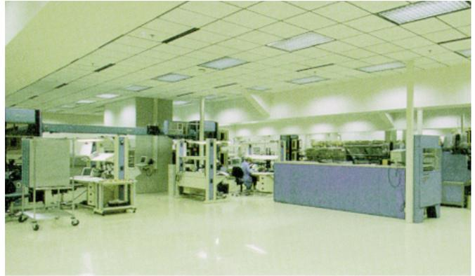
*In the circuit board assembly area at Allen-Bradley, a static dissipative floor helps ensure product quality.*
