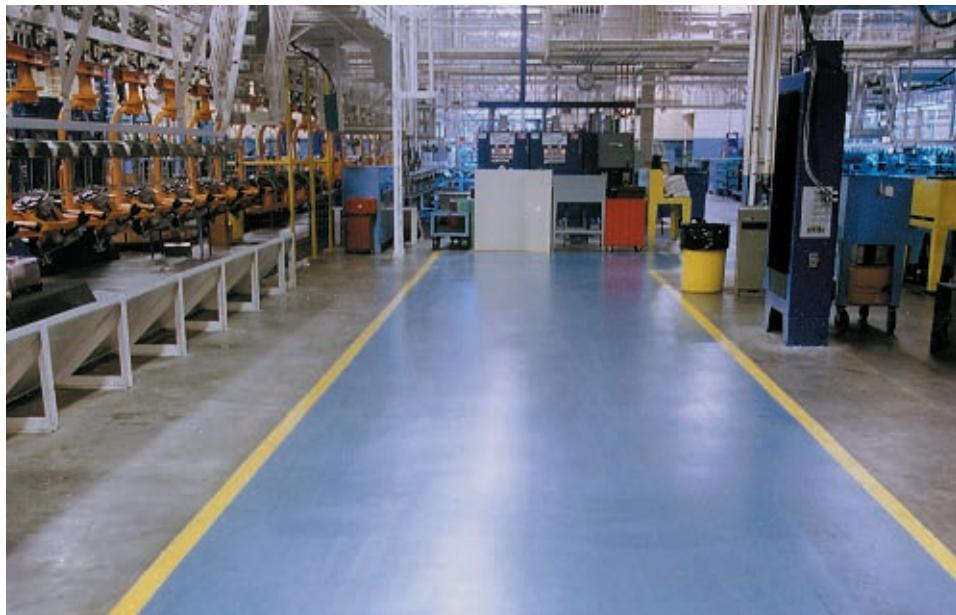
*Traffic aisle overlaid with Stonhard's Stonclad PT high-performance polymer flooring system provides a monolithic surface that's easy to clean and maintain. And, with an optional texture, provides a high level of slip-resistance for employee safety.*
